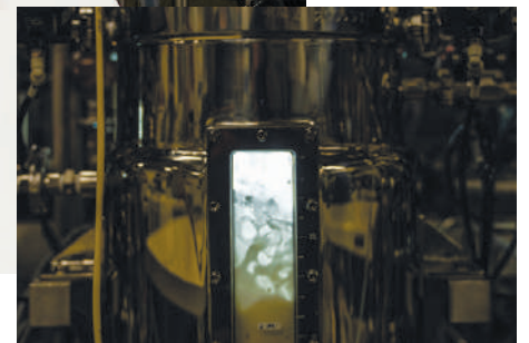
In a cultivation device, microorganisms are activated through constant agitation of the liquid fermentation medium.
