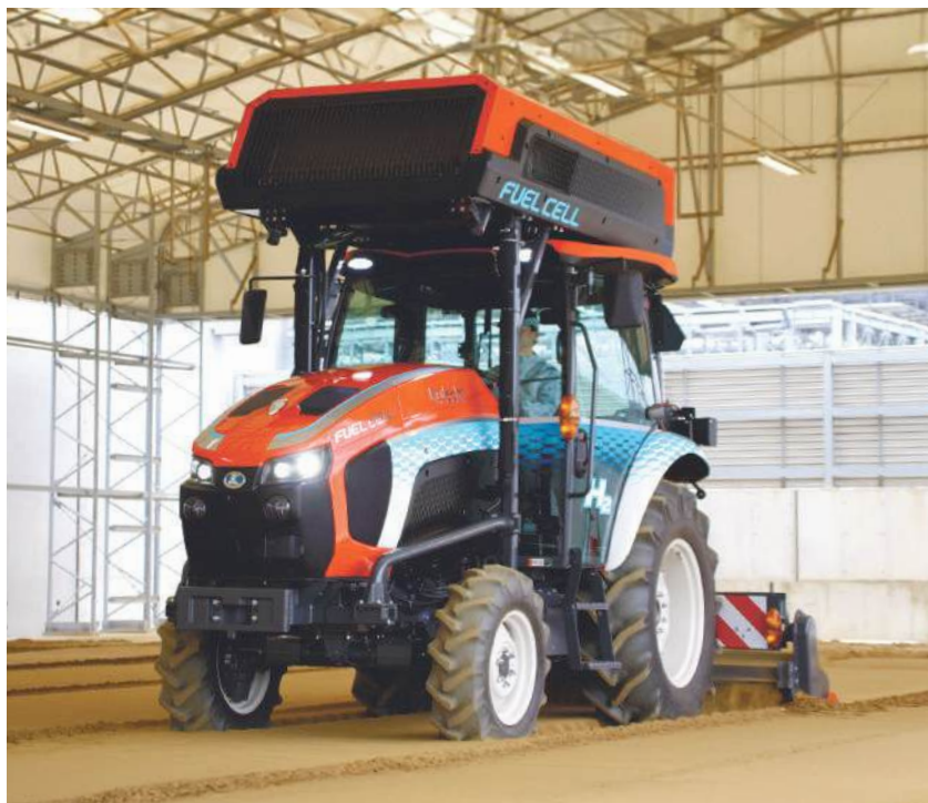
Kubota’s tractor with electric motors powered by fuel cells
